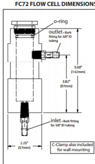
**SENSOR AND FLOW CELL INSTALLATION DIMENSIONS**
