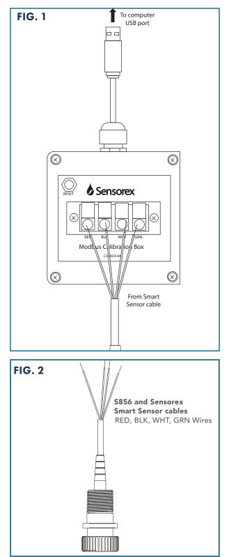
Products covered by this manual: S856 Cable assmebly, S272CD-MA and -MB, ICTS3020, FCL-MA and MB, CLD-MA and MB, and DO64000-MB NOTE: Not compatiblie with Sensorex ODO series
