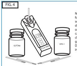
Note: The DPD method for measurement is not selective for chlorine dioxide alone. Other oxidants in the water can also be measured as chlorine dioxide. Using glycine strips prior to the DPD-1 strips removes interferences.
