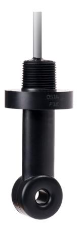
The Sensorex TCS series toroidal (inductive) conductivity sensors feature wide measurement ranges and dependable toroidal technology over the range 0-2000 ms/cm. Resistant to corrosion, coatings, and fouling common to contacting conductivity sensors, the TCS series is designed for a long and trouble-free service life.
